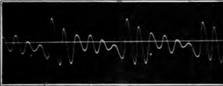
FIG. 108. Photograph of the vowel a in father , intoned upon the pitch n = 159 .
